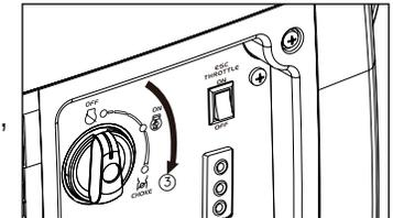
**TIP:** The choke is not required to start a warm engine. Push the choke knob in to the position “ON”.
