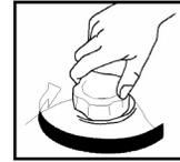
Remove the fuel tank cap by turning it counterclockwise.
