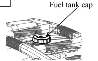
**Be sure the fuel tank cap is tightened securely.**
