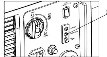
The overload indicator light (1) comes on when an overload of a connected electrical device is detected, the inverter control unit overheats, or the AC output voltage rises. Then, the AC protector will trip, stopping power generation in order to protect the generator and any connected electric devices. The AC pilot light (Green) will go off and the overload indicator light (Red) will stay on, but the engine will not stop running.
