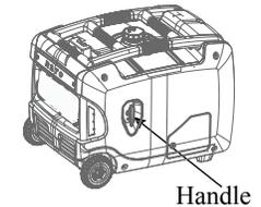
**TIP:** Grasp the carrying handle firmly to prevent the generator from falling over when pulling the recoil starter.
