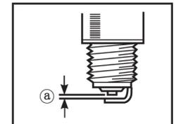
**TIP:** The spark plug gap should be measured with a wire thickness gauge and, If necessary, adjusted to specification.
