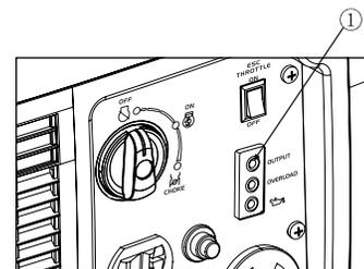
The AC power indicator (1) comes on when the engine starts and produces power.
