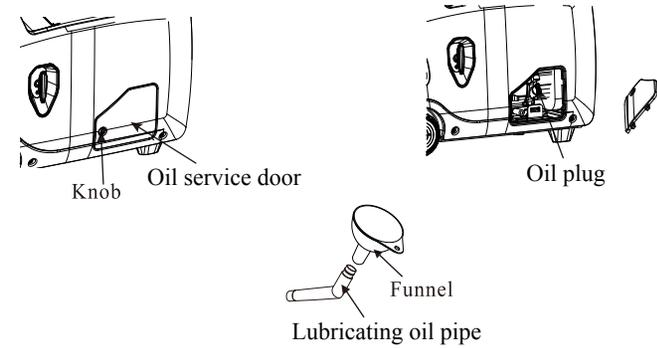
3. Unscrew the oil plug and then screw the sealing screw into the pouring orifice. Use the funnel to aid the specified amount of oil.
