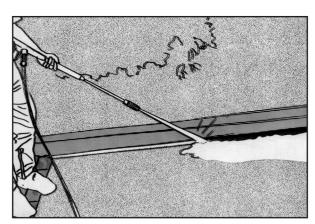
Adjust the vario to a zero degree stream. The pinpoint stream of water can be used to clean cracks, and narrow spots that are otherwise hard to reach. This concentrated stream can clean the toughest dirt spots.
