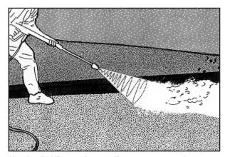
Use the dirt killer nozzle to act like a water powered sweeper. Let the power of the swirling nozzle push the dirt and debris. Acts like a water powered leaf blower.
