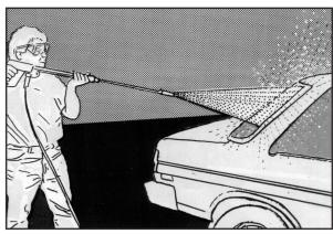
Clean by applying soap and rinsing it off with the vario nozzle. Just push the vario forward to have the soap injector begin applying soap. Then push it back to start the high pressure rinse. Wash your car, house or deck quickly without changing nozzles.
