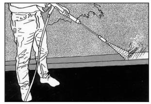
Rotate the cover of the vario to adjust the angle of the fan spray to get a narrower fan for greater cleaning power. Clean wood surfaces like curbs, decks, fences. No need to change nozzles just adjust the vario to apply soap and rinse.
