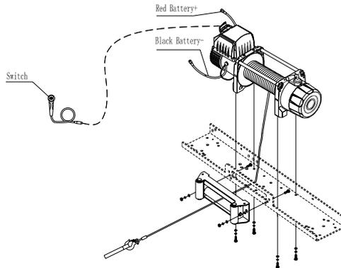
1. Your 12000lb winch is designed with a bolt pattern that is standard in this class of winch. Many winch mounting kits are available that utilize this bolt pattern for the most popular vehicle and mounting channels. If you cannot find a kit locally, contact us and we will provide you with the name of a dealer near you. If you will utilize the mounting channel you must ensure that it is mounted on a flat surface so that the three major sections (motor, drum and gear housing) are
