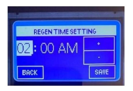
Use the + or – button to change time and press SAVE. Then press BACK three times to get back to MAIN MENU.
