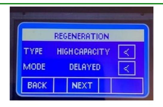
"MODE" toggles between DEMAND (factory setting) and DELAY. Delay lets the unit follow the time of day and then regenerates at the time selected.
