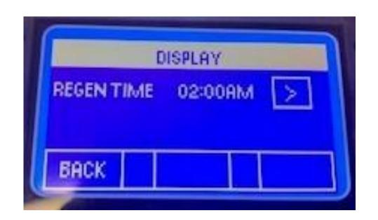
Here you can set the regeneration time if desired. This is used if put into the "Delay" mode.
