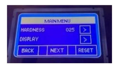
1<sup>st</sup> Screen when plugged in. At this point all you have to do set the hardness. Press the ">" symbol.
