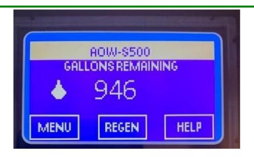
This is the screen that comes up when you touch the screen later on. (The screen goes off automatically and comes to life when touched.) It shows gallons remaining until regeneration.
