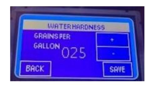
Press + or - button to adjust. Then press SAVE. At this point the unit is set. Just one setting and it's ready to go!!! Simple!
