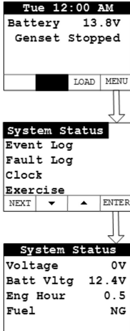
FIGURE 16. SYSTEM STATUS SCREEN
