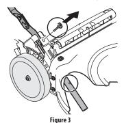
5. Pull upward on the handle (Figure 4) until holes in lower handle line up with holes in handle brackets (Figure 3 deck
