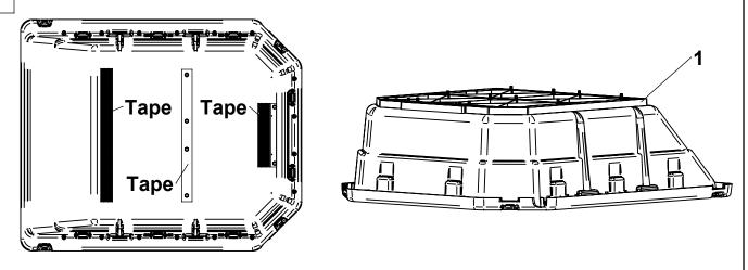
TIP: Bolt heads can be secured with tape to aid in asembly.
