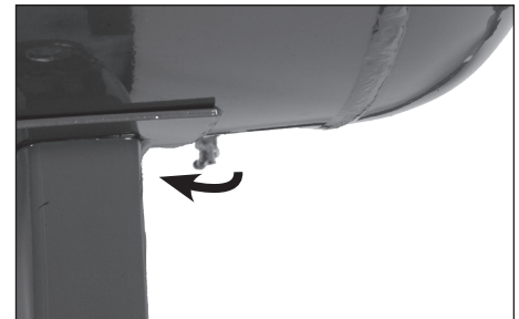
Figure 16 - Manual Tank Drain
