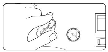
4. Pull the choke knob out to the "Choke" position.
