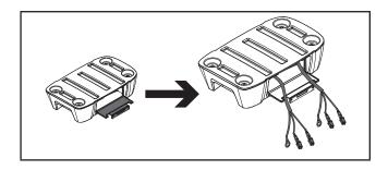
5. Plug one pair of power leads - connecting red to red and black to black (A), and ground wire (B) to inverter #1.
