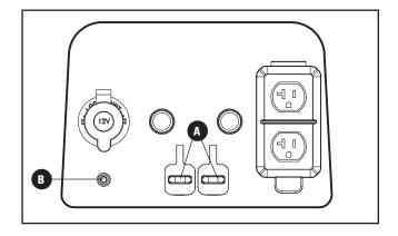
6. Plug the second pair of power leads connecting red to red and black to black (A), and ground wire (B) to inverter #2.
