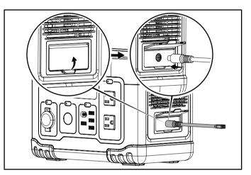
3. Plug the other end into a standard wall outlet. Ensure the cable is securely connected to the adapter.
