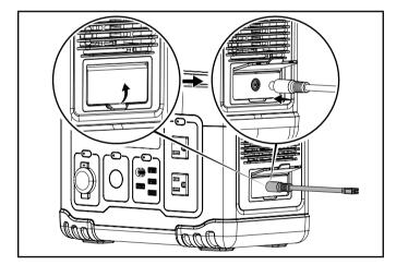
3. Connect solar panel using MC4 connectors.
