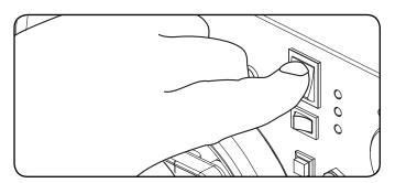
7. ELECTRIC START: Press and hold the ignition switch to the "START" position. Release as the engine begins to roll over. If the engine fails to start
