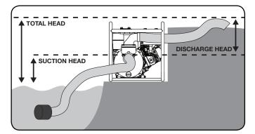
Pump output will be affected by the type, length, and size of the suction and discharge hoses. The pumping height, also known as the total head, is the distance from the water level to the point of discharge. As this distance increases, pump output decreases. The discharge capacity is greater than the suction capacity. Therefore, it is important that the suction head is less than the discharge head.
