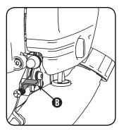
6. Push and release the primer bulb 5 times to prime the carburetor. You should see the bulb start to fill up with fuel and fuel traveling through the fuel line. (C)
