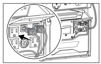
Connect one green and yellow grounding wire from the parallel kit to each Power Station by securing the ring terminal of the grounding wire between the nuts of the Power Stations grounding lug. Tighten the connection with a wrench.
