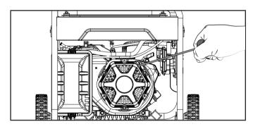
8. Move the choke lever to the "RUN" position.
