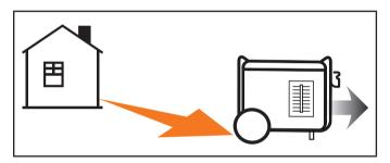
If misused and operated in an unapproved and unsafe location that results in the accumulation of poisonous CO gas inside an enclosed or partially enclosed space, for example a house, garage or a garage with the door partially open, CO Shield® will automatically shut off the generator and then will illuminate a blinking red LED light. **Read the action label for next steps.**
