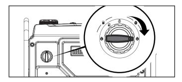
6. Move the choke lever to the "CHOKE" position.
