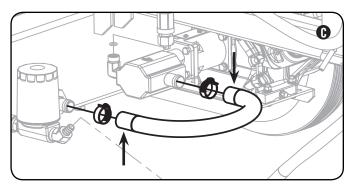
5. Using the provided d25 hose clamps, connect the hydraulic hose to the barb fitting on the control valve. Connect the other end of the hose to the barb fitting on the oil filter. (D)
