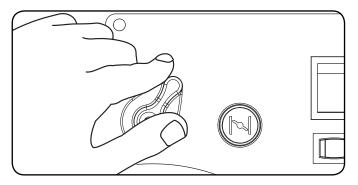
4. Pull choke lever out to the "Choke" position.
