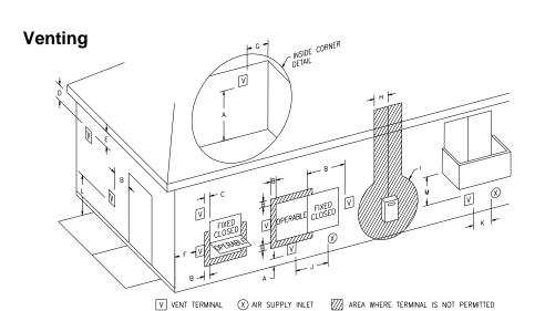
Figure 1 – Direct Vent Terminal Clearances
