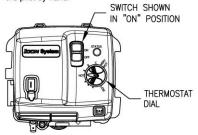
5. Slide the switch on the right side of the gas valve down to the "OFF" position
