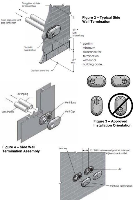
Figure 5 – Minimum Clearances: Multiple Side Wall Terminations
