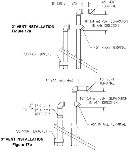
**NOTE:** For installations requiring both horizontal and vertical runs, the following rule must be followed: Total length of straight pipe (both horizontally and vertically) must **not** exceed the maximum equivalent length listed in these instructions.
