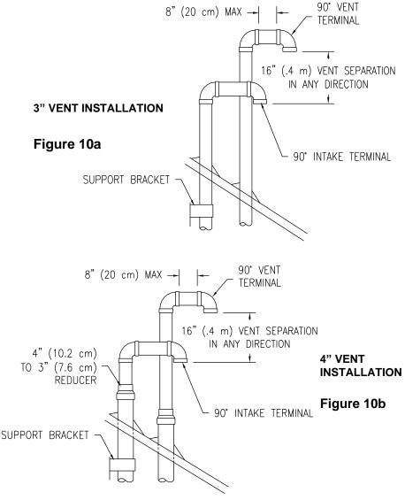
**NOTE:** For installations requiring both horizontal and vertical runs, the following rule must be followed: Total length of straight pipe (both horizontally and vertically) must not exceed the maximum equivalent length listed in these instructions.
