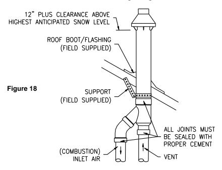
**NOTE:** For installations requiring both horizontal and vertical runs, the following rule must be followed. Total length of straight pipe (both horizontally and vertically) must not exceed the equivalent length listed in these instructions. For the concentric vent terminal, the maximum vent length is reduced by 10 ft.
