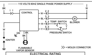
IF ANY OF THE ORIGINAL WIRES SUPPLIED WITH THE APPLIANCE MUST BE REPLACED, IT MUST BE REPLACED WITH APPLIANCE WIRE MATERIAL WITH A MINIMUM TEMPERATURE RATING OF 105°C AND A MINIMUM SIZE OF NO. 18 AWG.
