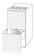
Make sure your HVAC cover panel is closed. Some systems will not turn on if the cover panel has not been closed properly.
