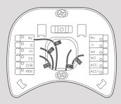
Insert your remaining wires into the side (not the front) of their corresponding terminal blocks.
