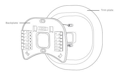
Pull the wires through the hole in the middle of the backplate and then attach the backplate to the wall using the drywall anchors and screws provided.
