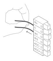
Check that all wires are properly inserted into the terminal blocks at the thermostat. Tug on the wires to ensure they are not loose.
