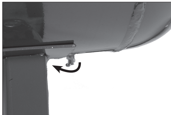
Figure 16 - Manual Tank Drain
