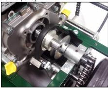
If there are any visible cracks, splits or gouges in the belt, replace it immediately. Also check the idler bearings regularly to ensure they spin freely and smoothly.
