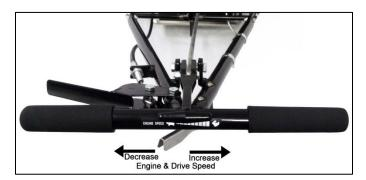
Pivot the lever right to increase, to the left to decrease On some units, the throttle also controls the engine stop switch as indicated previously.
