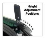
\*\*NOTE: Position #8 is not accessible in the unit's present configuration. Actual cutting height is affected by many
