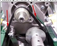
When the clutch lever is disengaged, the belt should sit just above the engine drive pulley, and should not spin. The belt guard and belt guide should slightly pinch the belt, ensuring that the belt rises above the influence of the engine drive pulley
