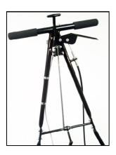
5. Attach the throttle cable wire to the engine's throttle control bracket as shown.
