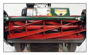
The mower is pre-set at the factory, but based on the type of grass and other factors, further adjustment may be necessary. As the blade reel and bed knife wear, additional adjustment will be required.
