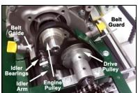
("clutch") is belt driven. When activated by squeezing the clutch lever on the handlebar, the belt simultaneously provides drive to both the reel
