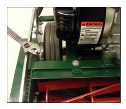
Turning the adjuster <u>clockwise reduces</u> the clearance between the bed knife and reel blade, while turning it <u>counter-clockwise increases</u> the clearance. When properly adjusted, there should be slight contact between the reel blade and the bed knife.
