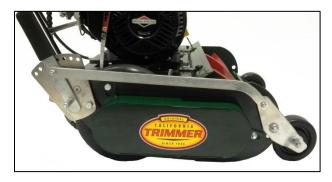
The front caster wheel axle comes standard in the middle position. It can be removed and placed in the bottom position to achieve additional settings and lower cutting heights. NOTE: the top position would be used only for aftermarket caster wheels or front rollers that prevent access to the lower cutting heights in the middle position.
