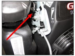
NOTE: Before tightening the cable holder, push the cable so that the throttle control activates (pushes in) the stop switch.
