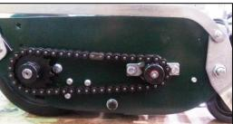
D. Check roller chain tension once each week. To tighten roller chain raise the roller aligning the roller shaft parallel to the drive shaft. This puts the roller at the furthest point of movement. Loosen the u-bolts and set screw on each side then move the roller back evenly until there is 1/2" vertical movement of the chain. Make sure the roller spacing is even across the back (with the yoke) and that the chain alignment is straight to the shaft sprocket. Tighten the u-bolts and set screws.
