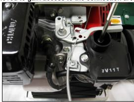
NOTE: Before tightening the cable holder, push the cable so the throttle control is in the slow position as indicated on the engine.
