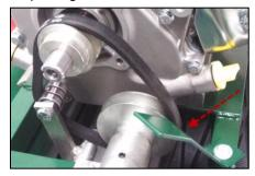
Remove cover, loosen belt guard and pivot away from belt. Remove belt from engine pulley, drive pulley and idler.
