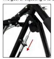
properly engages and disengages the drive system. Usually this can be done using the adjustment at the handle where moving it downward (in the bracket) will move the idler arm forward.
