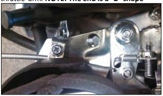
Step 3 – Remove Clutch Cable – Handle Side Remove the bolt, nut and spacers from the lever, then loosen the cable adjustment nuts so it can be removed from the bracket
