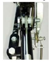
the first spacer, the cable end, the second spacer then the back side of the lever as shown in the picture.
