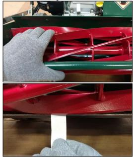
**NOTE: Excessive contact will cause overheating and damage to the parts.** Insufficient contact will not allow for the grass to be cut. Any excessive noise means that the adjustment is too tight. It is not recommended that the reel be engaged for extended periods of time when not cutting grass as the moisture provides a level of lubrication to the cutting surfaces while in use.
