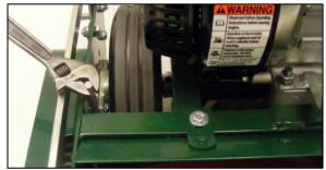
With the unit tipped back slightly and secured in place, the blade /bed knife contact can be checked by manually rotating the blade forward and use a narrow strip of paper to check the cutting action.
