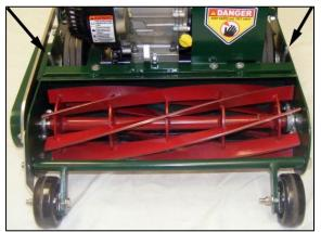
The adjusters raise and lower each side of the bed knife in relation to the reel, increasing or decreasing the clearance and should be moved as evenly as possible. Turning the adjuster <u>clockwise reduces</u> the clearance between the bed knife and reel blade, while turning it <u>counter-clockwise increases</u> the clearance. When properly adjusted, there should be <u>slight contact between</u> the reel blade and bed knife across the full width.
