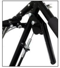
When disengaged, the belt tension is loose and it is in contact with the belt guide and belt guard to help prevent it from turning. If needed, the belt guide can be rotated to have more contact with the belt.
