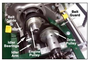
The drive belt is a wear item so some adjustments will be needed to maintain optimum performance. If there are any cracks, splits or gouges in the belt, replace it immediately. Also check the idler bearings to verify they spin freely and smoothly.
