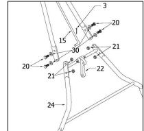
2. Attach the roller lift rod (#15) to the toggle (#22) using the co
