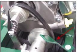
Remove nut, belt guide, 1 washer and 1 bearing from idler to create space to remove belt. Install new belt, re-assemble idler components and tighten with belt guide in proper position as shown.
