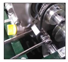
Verify belt is routed correctly and properly placed in the engine pulley and drive pulley. Move belt guard back into position and tighten. Squeeze the engagement lever to verify function. Reinstall the cover and tighten.
