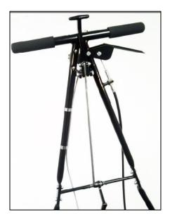
IMPORTANT: Check the movement of the throttle on the engine verifying that it travels freely and completely to the slow and fast positions when moving the lever.
