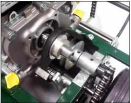
NOTE: When engaged (clutch lever fully squeezed), the belt guard and belt guide must not contact the belt.
