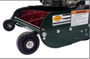
The height is changed by moving the adjustment handle into the positions of the bracket.
