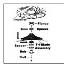
Loosen and remove the center bolt to disassemble the components. Placing all 3 of the spacers ABOVE the triblade assembly will provide the lowest cutting height, while placing 2 spacers below will provide the highest cutting height.
