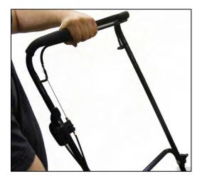
c. Place your foot on the deck and tilt the unit towards you while pulling the recoil starter.
