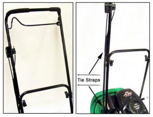
4. Verify that the engine stop lever is installed and it pivots upward completely against the handle.
