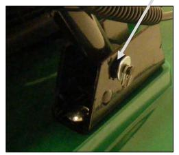
Attach the upper handle section to the lower handle section using the bolts and knobs. Fasten the corrugated tubing (which covers the throttle and engine stop cables) to the handles using the tie straps included.
