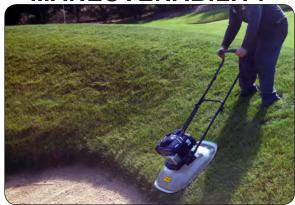
This lightweight yet powerful hover mower floats on a cushion of air and is designed to provide excellent cutting performance at angles up to 45 degrees for a wide variety of commercial, golf course and residential applications. It's extremely maneuverable as it glides over grass surfaces and it mulches as it cuts so the fine pieces fall easily to the soil surface.
