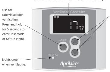
Use to override the calculated ventilation time setting (6–60 minutes/hr). Press and hold ▼ to turn ventilation OFF.
