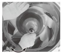
Turn this way to tighten. Turn this way to loosen. (The same directions as the fan rotation.)
