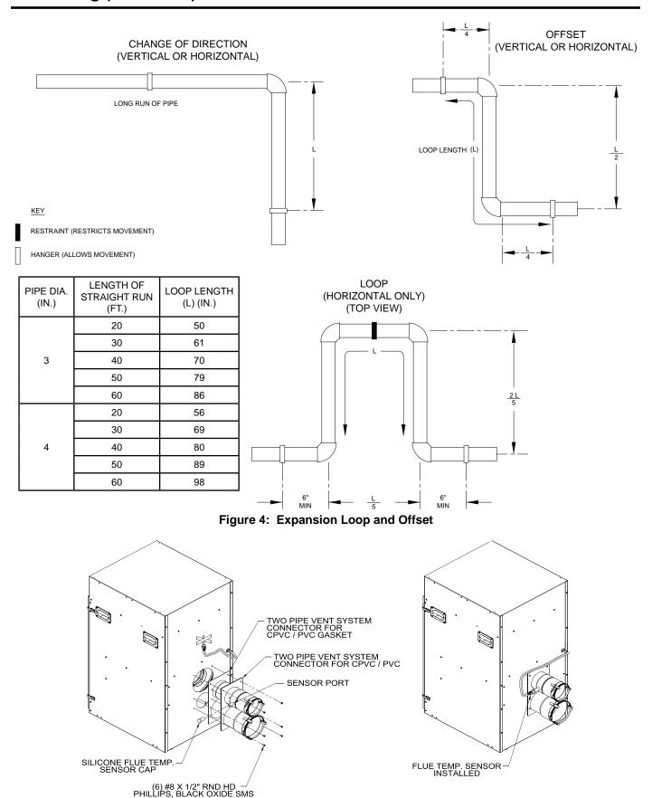
Figure 5: Field Installation of CPVC/PVC Two-Pipe Vent System Connector - Floor Mounted Boiler Builds
