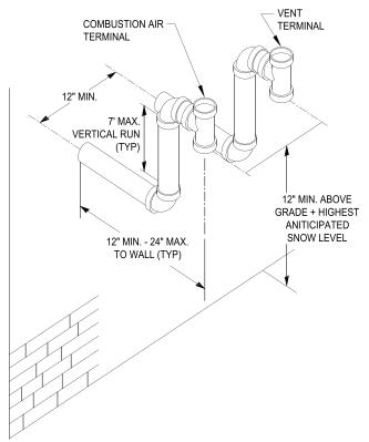
Figure 10: Direct Vent - Optional Sidewall Snorkel Terminations
