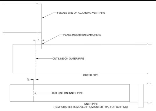
Figure 17: Cutting Straight Pipe
