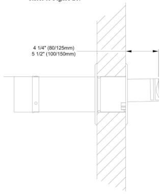
Figure 20: Horizontal Concentric Venting
