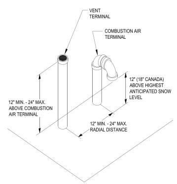
Figure 11: Direct Vent - Vertical Terminations
