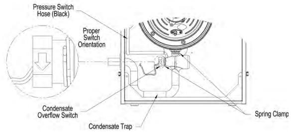
Figure 59: Condensate Overflow Switch Orientation
