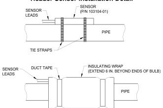
Figure 49: Alternate "Strap-on" type Header Sensor Installation Detail
