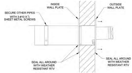
Figure 23: Completing Horizontal (Wall Terminal Installation)
