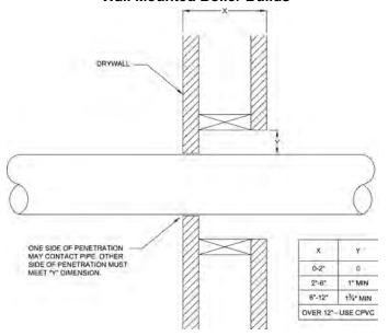
Figure 7: CPVC/PVC Vent Pipe Thru Combustible Wall Installation
