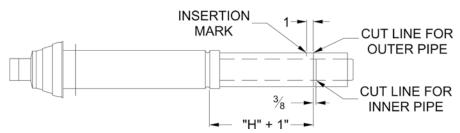
Figure 26: Cutting Vertical Terminal
