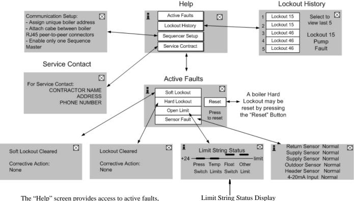
The "Help" screen provides access to active faults, lockout history, the service contact and the boiler reset button. The "Help" screen is accessed from the "Home" screen.
