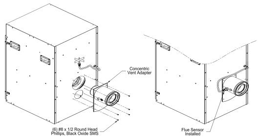
Figure 14: Field Installation of Boiler Concentric Vent Collar
