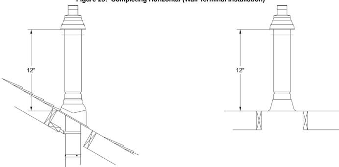
Figure 24: Vertical Concentric Vent Installation
