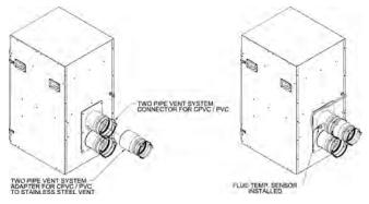
Figure 13: Field Installation of Two-Pipe Vent System Adapter for Stainless Steel
