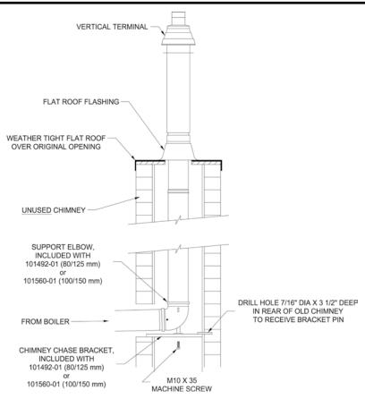
Figure 28: Chimney Chase Installation
