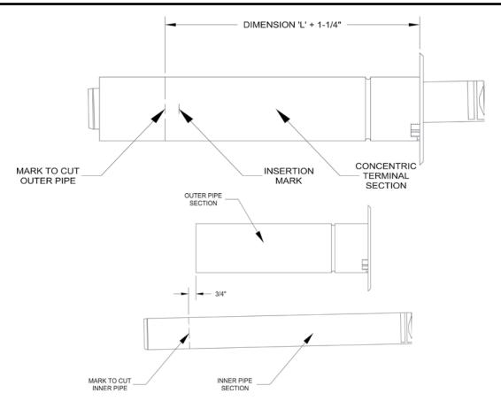
Figure 22: Cutting Vent Terminal Pipe
