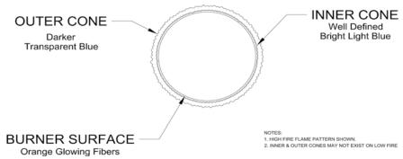
Figure 52: Burner Flame
