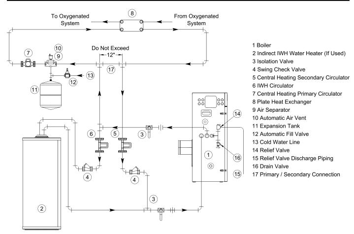
Figure 33: Isolation of the Boiler From Oxygenated Water with A Plate Heat Exchanger
