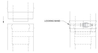
Figure 19: Joining Non-Cuttable Pipe
