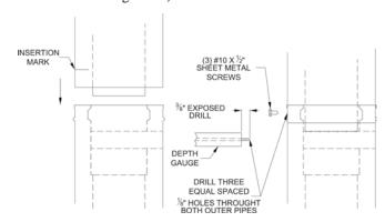
Figure 18: Joining Cuttable Pipe
