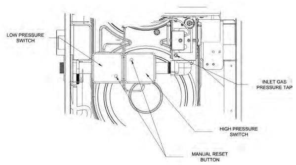
Figure 34B: Gas Inlet Pressure Switch Location
