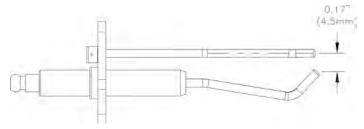
Figure 58: Ignitor Electrode Gap
