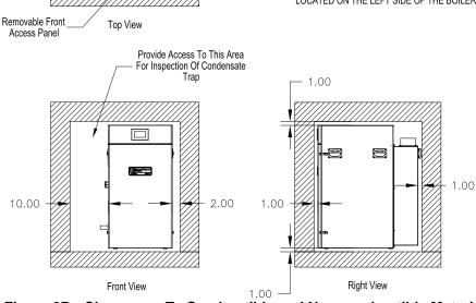
Figure 2B: Clearances To Combustible and Non-combustible Material, Wall Mounted
