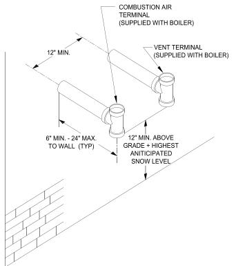
Figure 8: Direct Vent - Sidewall Terminations
