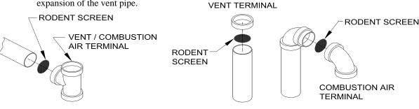
(B) VERTICAL Figure 9: Rodent Screen Installation
