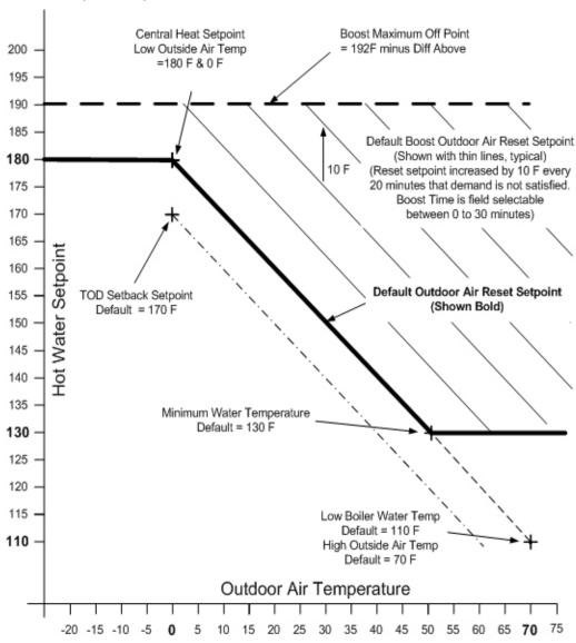
Figure 57: Outdoor Reset Curve
