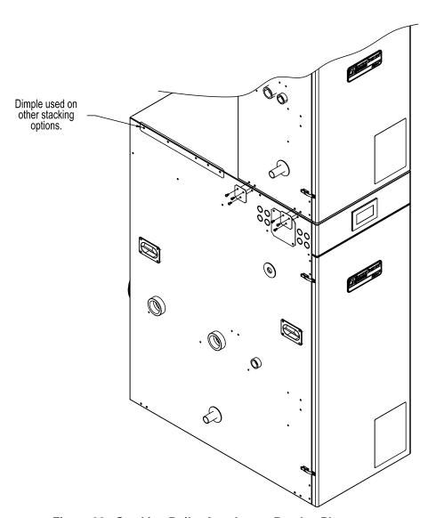
Figure 38: Stacking Boiler Attachment Bracket Placement
