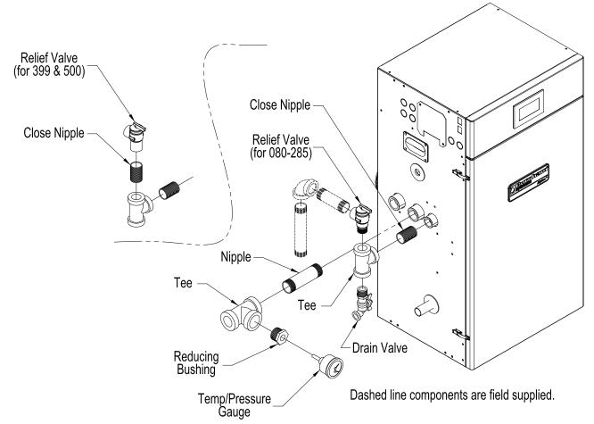
Figure 30: Factory Supplied Piping and Trim Installation
