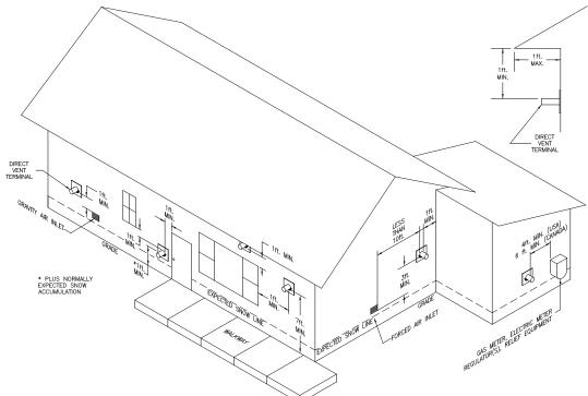
Figure 3: Location of Vent Terminal Relative to Windows, Doors, Grades, Overhangs, Meters and Forced Air Inlets (Concentric Terminal Shown - Two-Pipe System Vent Terminal to be installed in same location - Two-Pipe System Air Intake Terminal Not Shown)
