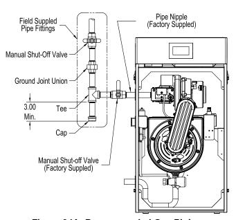
Figure 34A: Recommended Gas Piping
