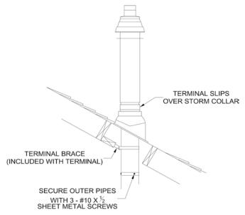
Figure 27: Completing Vertical Terminal Installation
