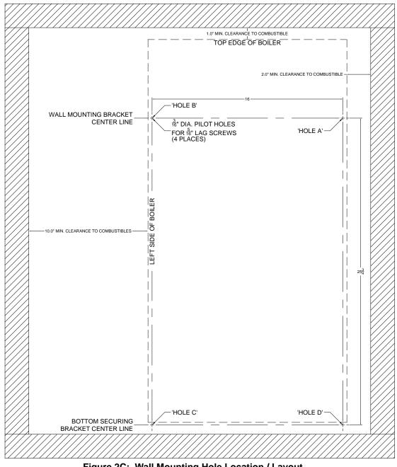
Figure 2C: Wall Mounting Hole Location / Layout
