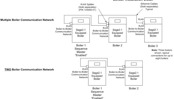
Figure 50: RJ45 Splitter Installation Detail
