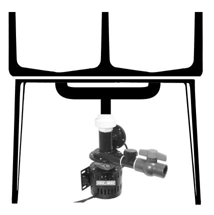
For installation on a twin laundry tub, the pump has to be centered as per this diagram.
