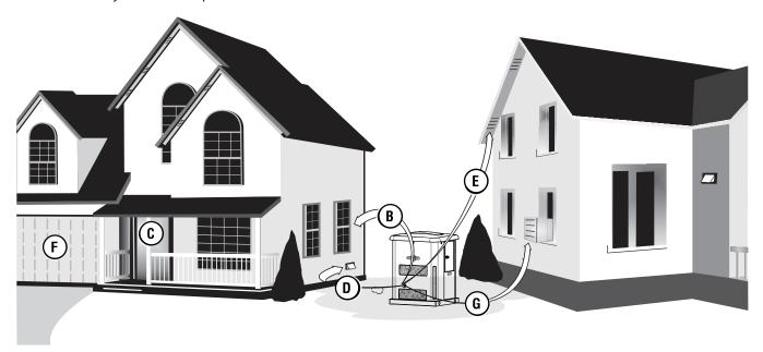
All fossil fuel burning equipment, such as standby generators, contains carbon monoxide (CO) gas in the engine exhaust. CO gas is odorless, colorless and tasteless and is unlikely to be noticed until a person is overcome. CO gas can kill you so it is required that the following is included as part of the installation:
