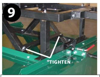
9. Tighten bolts on cross bar from Step 7.
