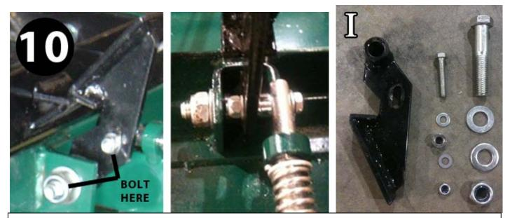
10. Install slam latch hook by aligning the angle of latch to the striker on the bed rest. See pictures above for proper hardware order. Tighten small bolt from hook to spring loaded pin only tight enough so hook and pin still move freely. Use hardware labeled I.
