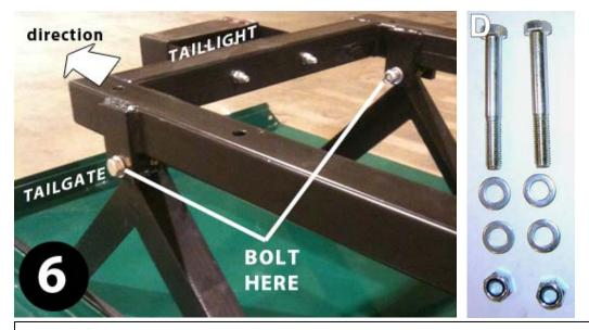
6. Take assembly portion from **STEP 5** and install to struts as shown in photo above, with the taillight pointing toward the tailgate. Use pivot bolts from package labeled D.
