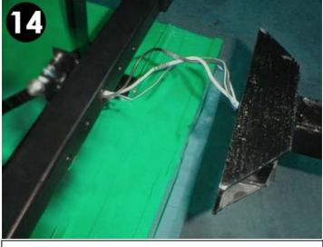
14. On the tongue assembly, connect the male electrical connectors to the female electrical connectors, ensuring that the colors of the wires match. BE CAREFUL NOT TO DAMAGE WIRES.
