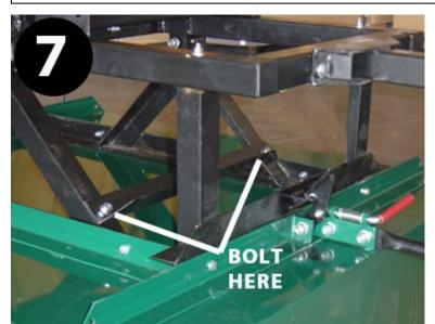
7. Install cross bar to the struts with direction of 'angle iron' on the bottom as shown, use bolts from package labeled EX. **Leave bolts loose**- do NOT tighten until Step 8.
