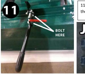
11. Install handle to the bed as shown in the photo left. Use hardware labeled J.
