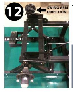
12. Mount idler axle to the frame with the swing arm pointing to the rear or taillight, use bolts from package labeled H.
