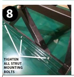
8. Tighten bolts that join bed and sub frame struts from Step 4.
