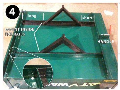
4. Mount subframe struts with shortest section of struts closest to the handle, photo left. Each strut is either *Right* or *Left*. Place each strut on the inside portion, flush with the bed, use bolts from package labeled AX.
