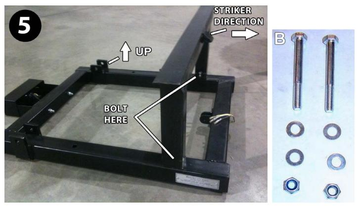
5. Install bed rest to rectangular frame as shown in the photo above with the Striker pointing forward, use bolts from package labeled B. Notice the direction of the pivot point near the taillight points up in the same direction as the mounted bed rest.
