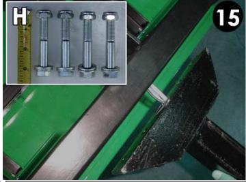
15. Install the tongue assembly to the frame. Tighten to 50-71 ft-Ibs (68-96nm). Be sure the wires do not become pinched between the frame and the tongue. Use bolts from package labeled H.
