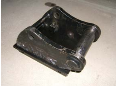
Figure 11: Mounting plate with excavator attachment
