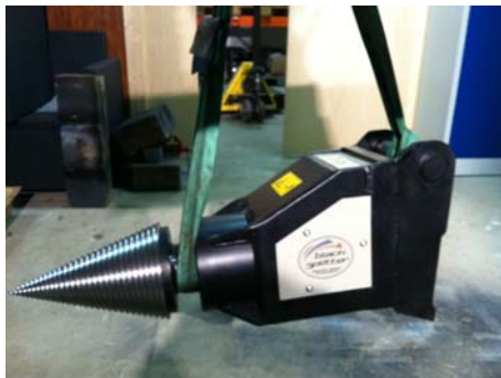
Figure 9: Lifting straps on the Black Splitter
