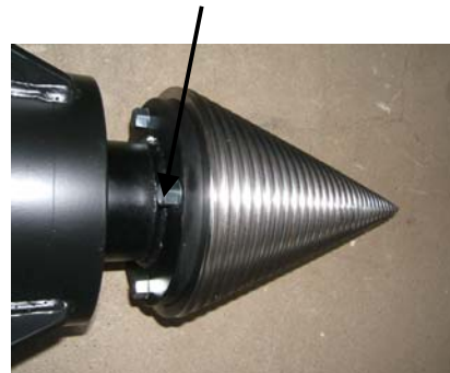
Figure 14: Screw cone mounted on the Black Splitter
