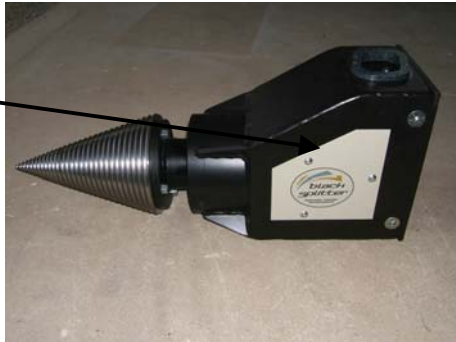
Figure 6: Side protective cover on Black Splitter
