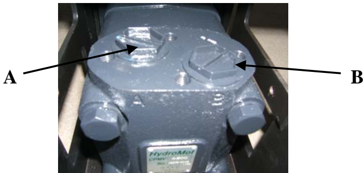
Figure 10: Connections of the hydraulic motor
