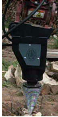
Figure 8: Black Splitter with excavator attachment
