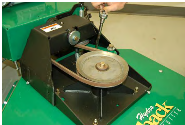
Removing tension on the blade belt
