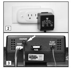
outlet is operating, but the "Power" warning light is still on, replace the charger unit with the Basement Watchdog part number 1015001 from Glentronics at 800-991-0466, option #3.
