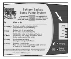
Check your security system to determine whether an open (no contact) or closed (making contact) connection is needed to activate the alarm.
