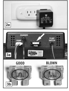
NEGATIVE (-) post, and then the RED wire to the POSITIVE (+) post. Tighten the wing nuts on the battery posts. (e) Plug the control unit back into the wall outlet.
