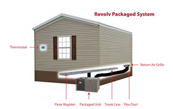
A **Revolv Packaged System** can provide both heating and cooling from one self-contained unit, placed outside of the home. Only air and electric connections must be made to connect the system to the home's prefabricated ductwork.
