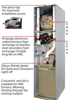
4 speed direct drive blower for quiet, efficient operation
