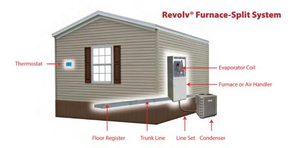
A **Revolv Split System** can provide both heating and/or cooling, that is split into two primary sections—outdoor and indoor. A complete HVAC system would consist of an indoor coil attached (installed in a pressurized compartment) to a Furnace/Air Handler installed in the home, and is connected to the outdoor condenser section by a refrigerant line set.
