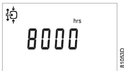
Example of running hours screen
