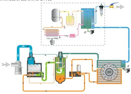
A Intake air B Air/oil mixture **C** Oil D Wet compressed air
