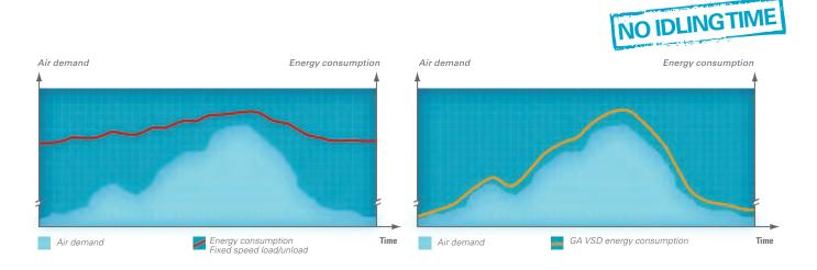
In almost every production environment, air demand fluctuates depending on different factors such as the time of the day, week or even month. Extensive measurements and studies of compressed air demand profiles show that many compressors have substantial variations in air demand.
