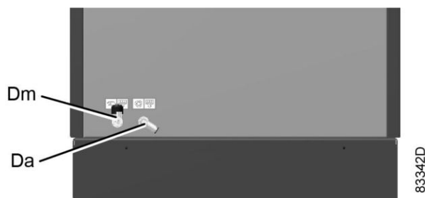
Condensate drain connections, GA Workplace
