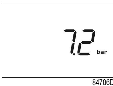
Main screen with pressure (stopped compressor)
