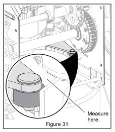
If roller is 12.7 mm – 22.2 mm (1/2" – 7/8") from frame, no further adjustment is required.
