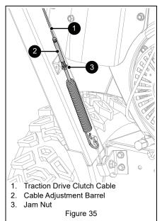
With the traction clutch disengaged, make sure auger idler arm lightly touches the frame. See Figure 36.
