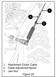
5. With the attachment clutch disengaged, make sure auger idler arm lightly touches the frame. See Figure 30.
