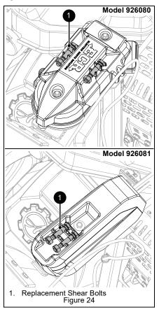
**IMPORTANT:** Ariens recommends using only Ariens OEM shear bolts when replacing shear bolts. See *Service Parts* on page 16.
