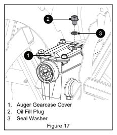
Check oil level with suitable measuring device, such as a clean screwdriver, and add oil if needed. Oil level must be 6.1 cm - 6.7 cm (2.4" - 2.6") from the flat surface of the gearcase cover.
