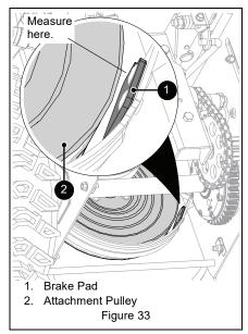
If there is less than 1.6 mm (1/16") gap, loosen idler adjustment nut and move idler away from belt or pulley. Position idler to achieve a 1.6 mm (1/16") minimum brake pad gap and a 12.7 mm – 22.2 mm (1/2" – 7/8") gap between the plastic roller and the frame. See Figure 32.
