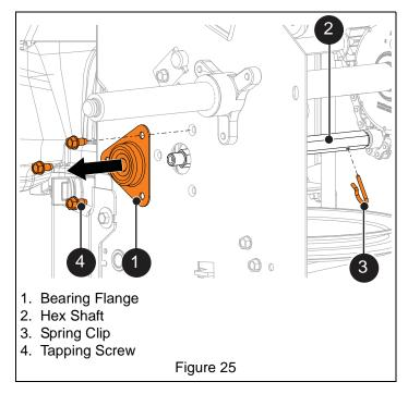
**NOTICE:** For track models, track angle must be in the "Lowered Position" to remove hex shaft. Refer to Operator's Manual. See Figure 26.
