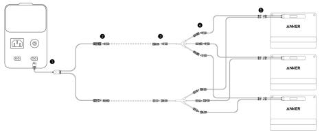
\*If the solar panel is far from the power station, you can purchase the Anker SOLIX Solar Panel MC4 Charging Cable as an extension cable from Anker's official website, and connect it to the part indicated by the dotted line in the diagram.
