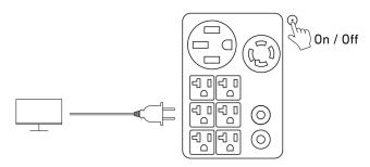
Double-click the AC outlet button, wait until the car icon appears on the screen, then connect your EV charge to the L14-30R or 14-50 AC output port.
