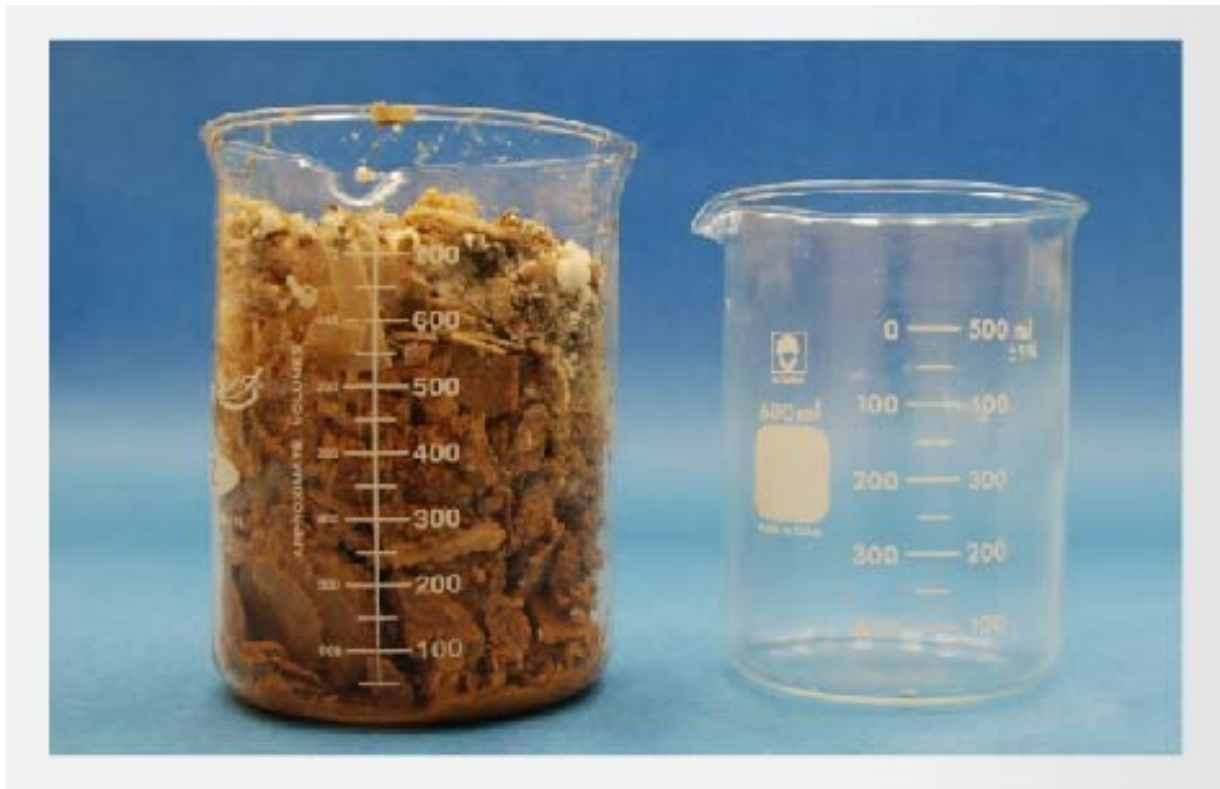
Figure 3: 1 liter or 320 g of scale deposit removed from Test Unit B (without ScaleRX®)
