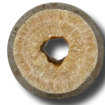
A cross-section of built up lime scale on the outlet of a water heater in Northern Illinois.
