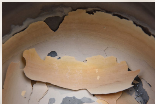
Water heater with scale and sediment buildup decreasing the efficiency, water pressure and lifespan of this water heater.
