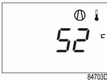
Main screen with temperature (stopped compressor)
