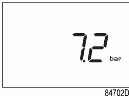
Main screen with pressure (stopped compressor)
