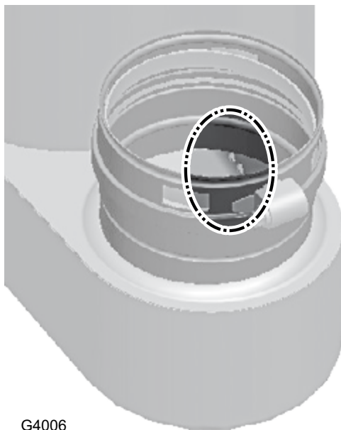
Figure 83 Recuperator flue way drain holes
