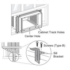
Carefully place the cabinet back in the window and align the cabinet track holes with the support brackets. Attach each support bracket to the cabinet through a cabinet track hole, using a type D screw and a lock nut. Use the first track hole past the sill bracket on the outer edge of the window sill. Tighten the lock nuts on the support brackets to secure them to the sill brackets.
