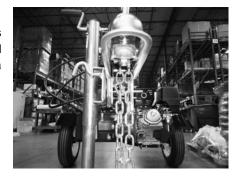
11. Place the hitch over the attachment tube, aligning the bolt holes, and insert the rear 1/2 x 3-1/2 inch bolt (A). Install and tighten the locknut.
