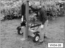
c. Turn the knob handle until the pin slides into the slot. This allows the plunger to snap into place, securing the rail assembly in a vertical position.
