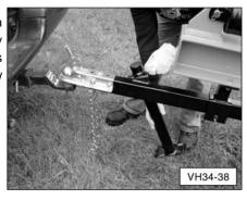
**4**. Attach the towing safety chains to the tow vehicle.
