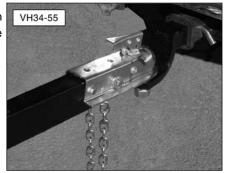
Raise the front leg to the towing position by pulling the spring pin. If not already secure, make sure the hitch coupler is properly and securely attached to the tow ball.
