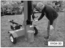
f. Hold the control lever, extending the splitting wedge, until the log is split or the cylinder rod stops at its maximum travel position. Stop the log splitter (forward movement), at any point in the splitting process, if you feel an unsafe log splitting condition is occurring. As the log is being split, DO NOT reach forward and attempt to catch the split wood — let it fall to the ground.
