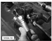
16. Attach the other high-pressure hose from the bottom valve fitting to the pump. Coat the threads of the fitting with a thread sealing material and securely tighten the hose fitting.
