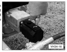
17. Remove the oil filter from the plastic cover and apply a thin coat of oil to the rubber seal. Screw the filter onto the filter head, located near the hydraulic tank. Once the filter makes contact with the filter head, turn it an additional 3/4 turn. Hand-tighten only.
