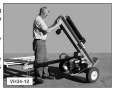
Link the ends of the safety chains together with the safety quick-link and tighten the link's locknut securely with a wrench.
