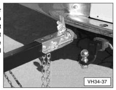
Release the latch assembly on the hitch coupler and lock the hitch coupler onto the tow ball.
