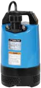
**LB-800 • LBT-800 Slimline design pumps** allow to fit into 8" pipes. Powerful pump built with durable materials in an easy handling design. Top discharge provides maximum motor cooling efficiency allowing continuous duty operation at low levels and extended dry-run capability.
