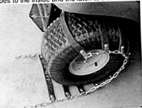
2) Drive onto the tire chains leaving approx. 2/3 of the chain in front of the tire and drape the long portion of the chain around the tire. Hook the inside first, starting with the very last link. Repeat with the latch side (outside).
